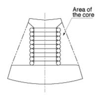
Fig.2 Rear view of the divided laminated core
