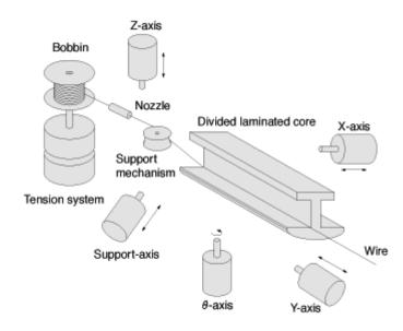
Fig.10 Process of wire winding
