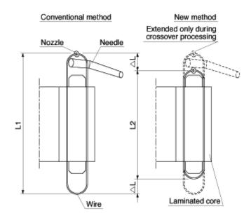
Fig.8 New work rotation type wire winding machine
